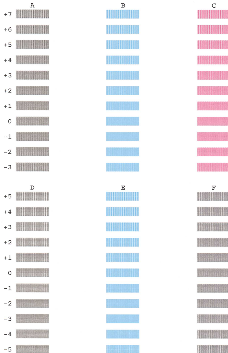
Figure 2-10 Printing Position Adjustment Pattern (S750/S520)
